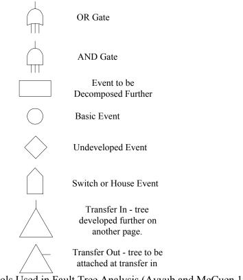
Figure 5. Symbols Used in Fault Tree Analysis (Ayyub and McCuen 1997)
