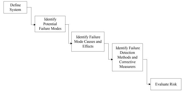
Figure 3. Failure Mode and Effects Analysis (FMEA) Process
