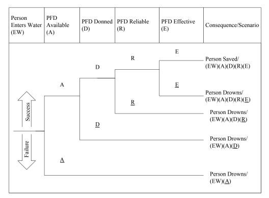
Figure 4b. Event Tree Example for a Personal Flotation Device
