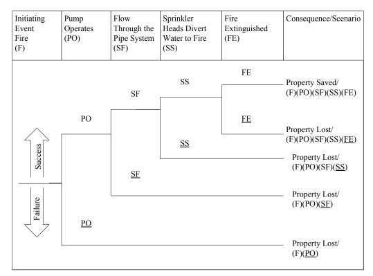
Figure 4a. Event Tree Example for Sprinkler System
