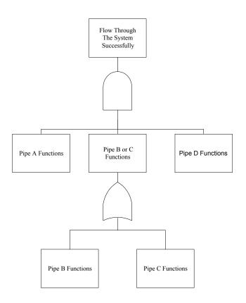
Figure 7a. Success Tree for Pipe System Example
