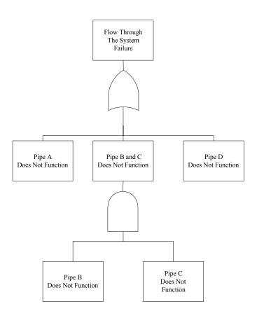
Figure 7b. Fault Tree for Pipe System Example
