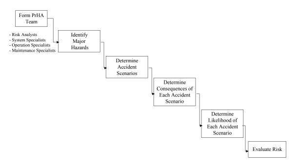
Figure 2. Preliminary Hazard Analysis (PrHA) Process
