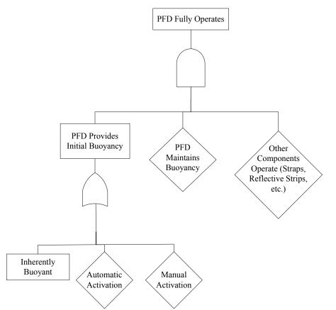
Figure 8. Success Tree for the Full Operation of a Personal Flotation Device
