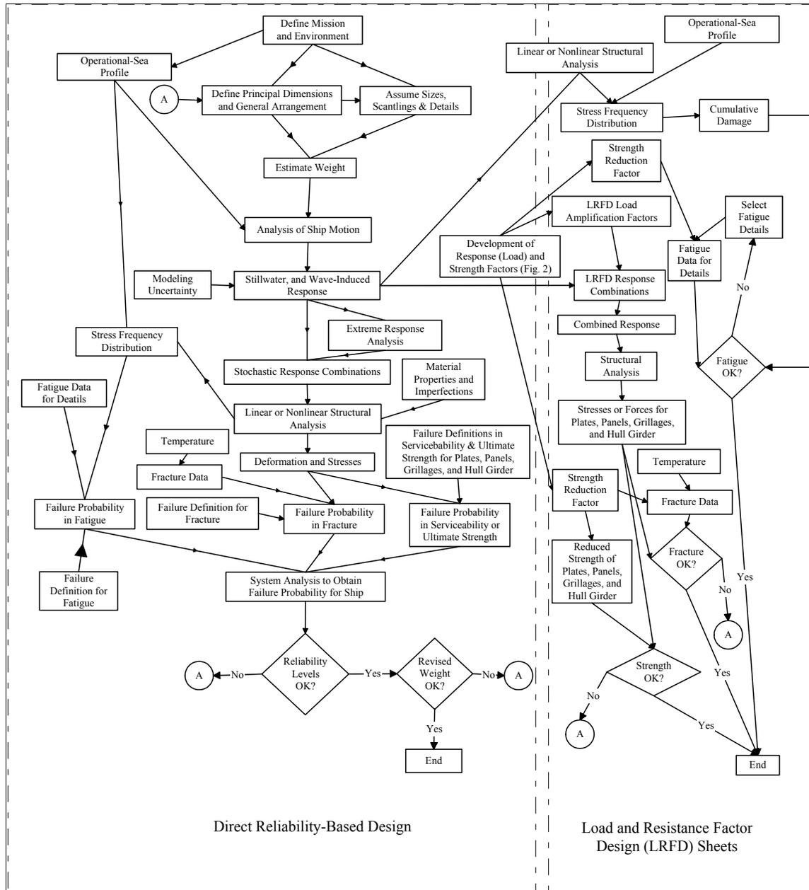
Figure 2. Reliability-based Design of Ship Structures (Ayyub et al 1999)
