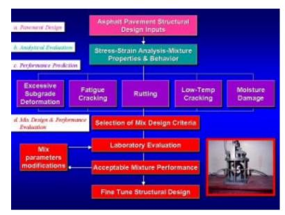
Performance Based Mix Design Methodology for Modified Asphalt Mixtures
