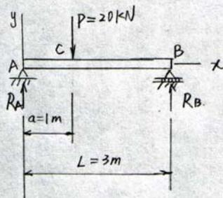
Equation of elastic curve for CB ( $a < x < L$ )
