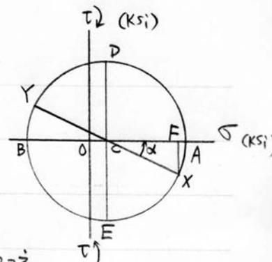
③  $\tan \alpha = \frac{FX}{CF} = \frac{FX}{OF - OC} = \frac{8 \text{ ksi}}{18 \text{ ksi} - 3 \text{ ksi}} = \frac{8}{15} = 0.5333$
