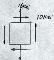
(a) stress  $\sigma_{x'}$   $\sigma_{y'}$   $\tau_{x'y'}$  when  $\theta = -25^\circ$   $2\theta = -50^\circ$
