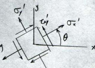
(b) stress  $\sigma_{x'}$   $\sigma_{y'}$   $\tau_{x'y'}$  when  $\theta = 10^\circ$   $2\theta = 20^\circ$
