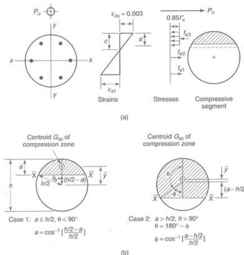
**Figure 19.** Circular Columns: (a) Strain, Stress and Compression Block Segment; (b) Compression Segment Chord  $x-x$  Geometry
