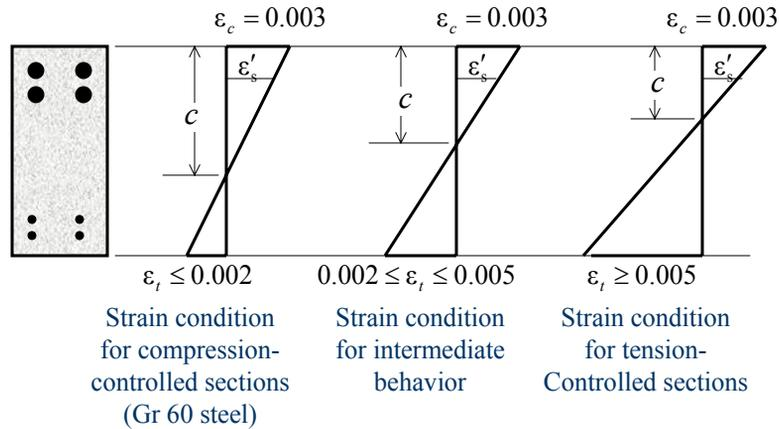
**Figure 7.** Stresses and Forces in Columns
