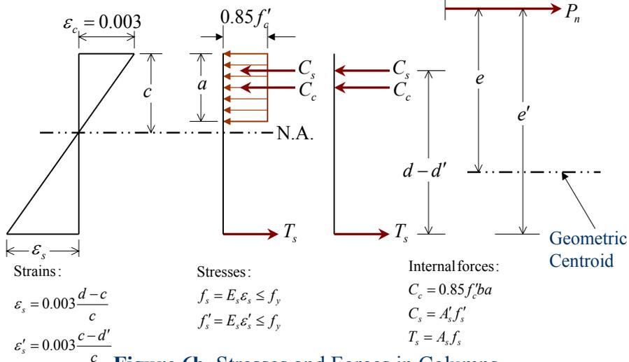
Figure 6b. Stresses and Forces in Columns
