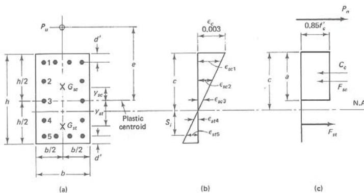
**Figure 18.** Column Reinforced with Steel on all Faces: (a) Cross-Section; (b) Strain; (c) Forces
