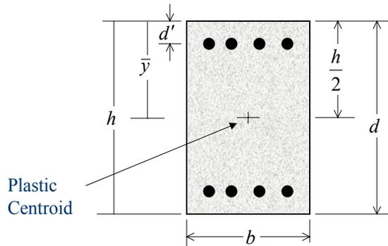
Figure 6a. Stresses and Forces in Columns
