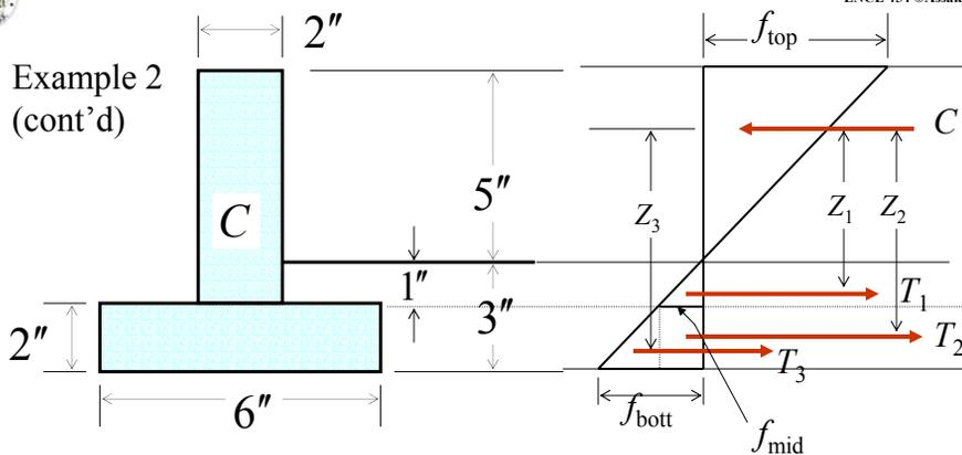
$$C = T = T_1 + T_2 + T_3$$
