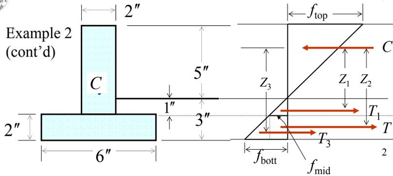
$$60,000 = 4\left(\frac{1}{3} f_{\text{bott}}\right) + \frac{16}{3}(4 f_{\text{bott}}) + \frac{17}{3}(4 f_{\text{bott}}) = \frac{136}{3} f_{\text{bott}}$$
