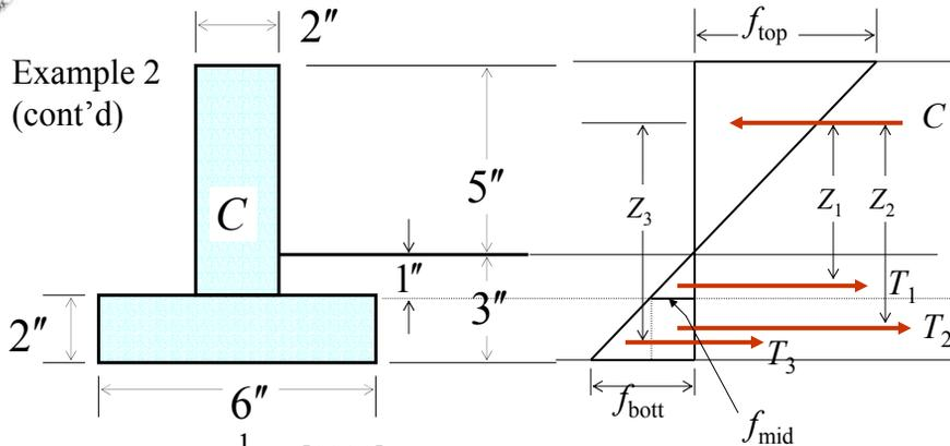
$$C = f_{\text{avg}} \times \text{area} = \frac{1}{2} f_{\text{top}} [(5)(2)] = 5f_{\text{top}}$$
