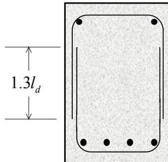
**Figure 9.** Overlapping U-stirrups to form a closed stirrups
