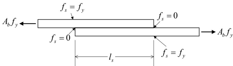
**Figure 10.** Stress transfer in tension lap splice
