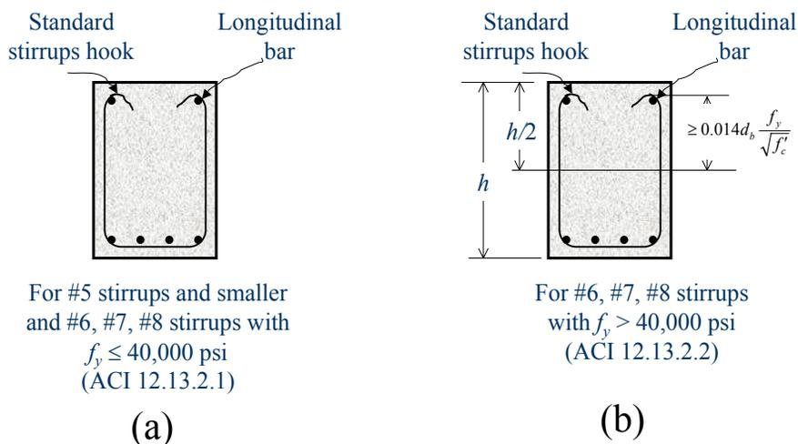
Figure 8. Web Reinforcement Anchorage
