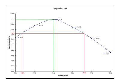
Maximum dry unit weight =  $105.79 \text{ lb/ft}^3$ Optimum moisture content = 14%
