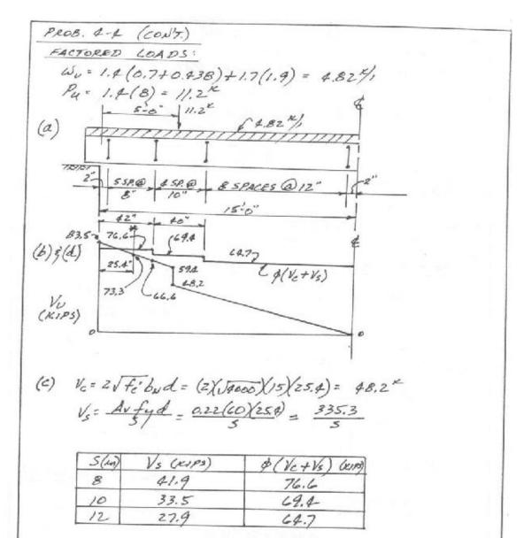
(d) NOTE THAT  $V_U < \phi(V_C + V_S)$  AT ALL LOCATIONS FROM THE CRITICAL SECTION (\*) TO THE & OF THE SPAN. (SEE ABOVE SKETCH DESIGNATED (b) 3(d).)
