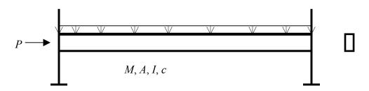
where  $\sigma$  = computed compressive stress, c = distance from the neutral axis to the extreme fiber, P = applied axial load, M = applied moment due to external loads, A = cross sectional area of the beam, I = centriodal moment of inertia of the cross section, and  $F_y$  = yield strength of steel. The variables c, P, M, A, I, and  $F_y$  are called basic random variables. The probabilistic characteristics of these variables are provided in the table shown below (Table 1).
